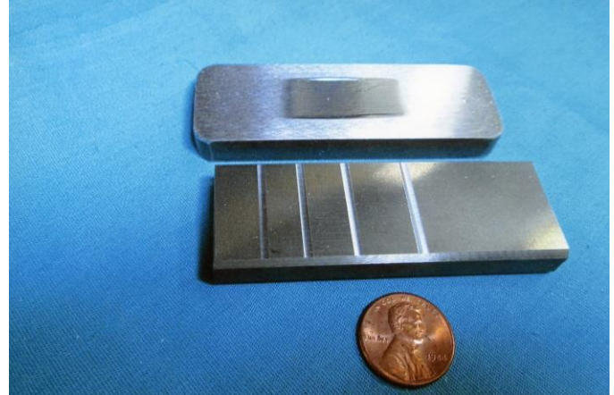
Figure 2 Four ASTM G174 abrasion tests on one ASTM G65 test specimen.
